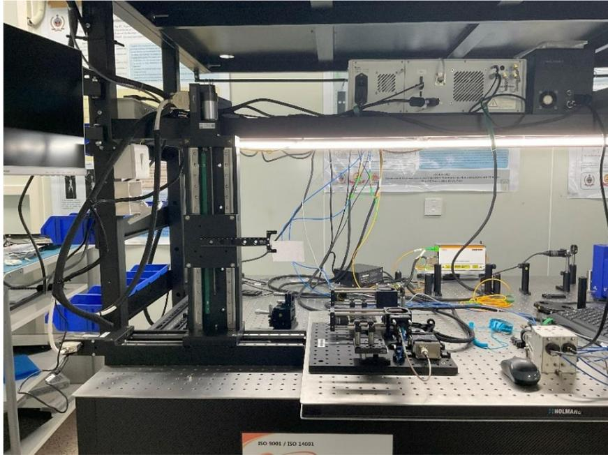
Figure :THz Spectroscopy cum Imaging System
